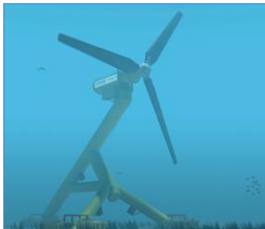
Figure 2.23: HS1000 Tidal Energy Device from Hammerfest Strom
