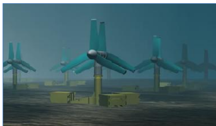
Figure 2.18: AK1000 Tidal Turbine from Atlantis Corporation
