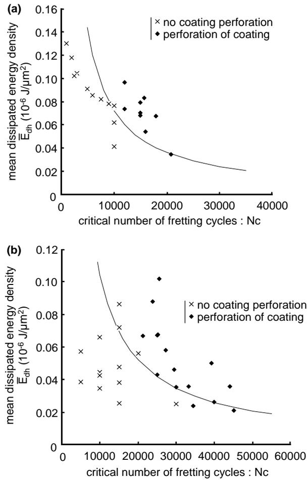
Figure 5. Durability estimation of (a) TiN and (b) TiCN coatings. Solid line corresponds to the mean coating endurance. Fretting test conditions:  $P=50\text{-}150\text{N}$ ,  $\delta=50\text{-}200\mu\text{m}$ ,  $RH=50\%$ ,  $f=5\text{Hz}$ .
