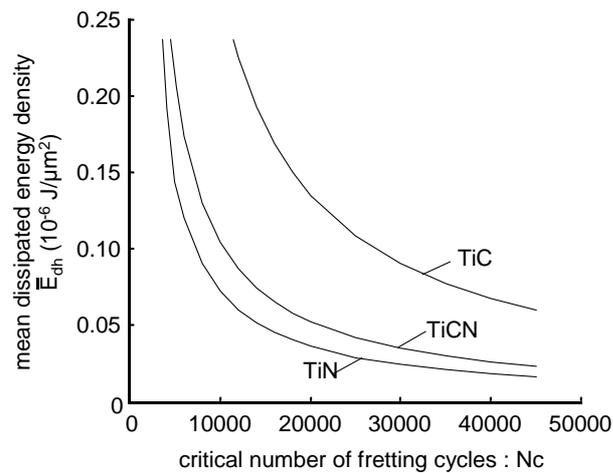
Figure 8. Durability of hard coatings as a function of the critical number of fretting cycles for different coatings with a given thickness: TiC-1.6μm, TiCN-2.5μm, TiN-4μm.
