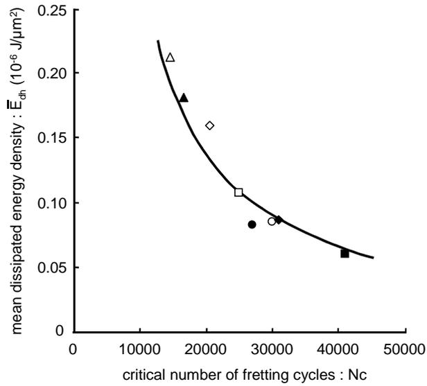
Figure 4. TiC coating endurance for different sliding amplitudes: constant ones (■ 50μm, □ 100μm, ◇ 150μm, Δ 200μm) and variable (◆ (50/100)μm<sub>x1</sub>, ○ (50/100)μm<sub>x2</sub>, ● (50/100)μm<sub>x4</sub>, ▲ (150/200)μm<sub>x1</sub>). Fretting test conditions: RH=50%, f=5Hz, P=100N [20].
