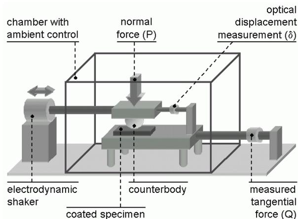
Figure 2. Schematic of the fretting rig.
