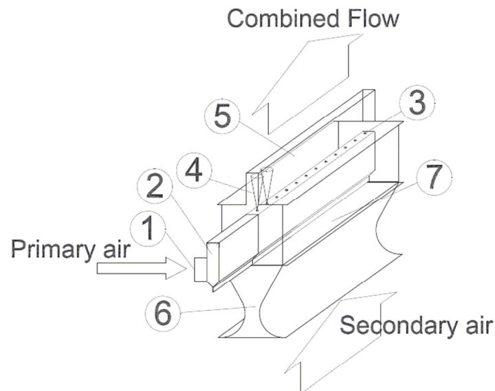
Figure 1. Construction of the induction measurement device.
