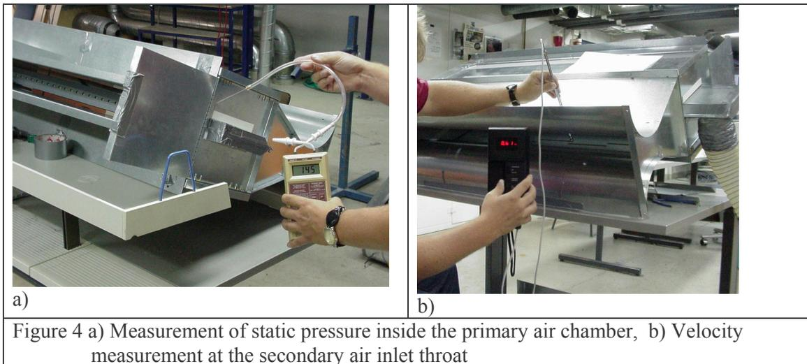
The primary air flow through the nozzles was calibrated using an orifice plate. Correlation between the measured flow rate at the orifice plate and measured static pressure in the chamber was established and used to determine the actual primary air flow rate.
