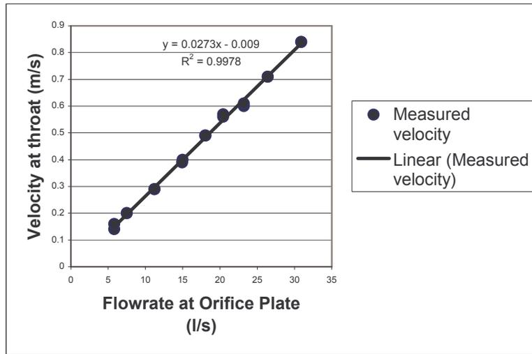
Figure 6. Correlation between throat velocity and volume flow.
