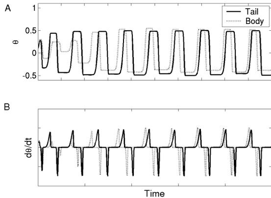
Figure 6: Two phase-lagged segments. Graph A shows the segment oscillations ( $\theta$  is in radians); graph B shows the input to the segments from their muscles DM and VM (equal to  $d\theta/dt$ ). The two segments oscillate approximately 9/10 of a cycle out of phase. An initial transient phase can be observed until the oscillations settle at a stable frequency and amplitude.
