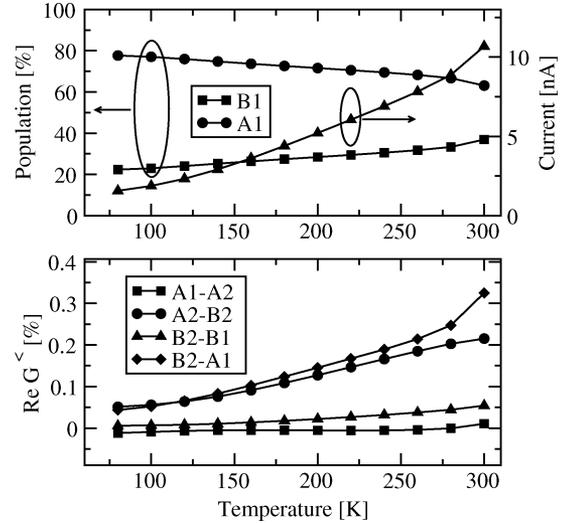
Fig. 3. Temperature dependence of populations of energy levels (top panel, left axis), current (top panel, right axis), and real part of coherences among states (bottom panel) at the field  $F = 32$  kV/cm.
