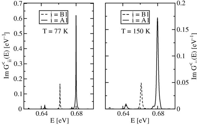
Fig. 4. Energy distribution of the population of the upper (full line) and lower (dashed line) laser level of the prototype of a QD cascade laser structure at the field  $F = 32$  kV/cm and temperatures of  $T = 77$  K (left) and  $T = 150$  K (right).
