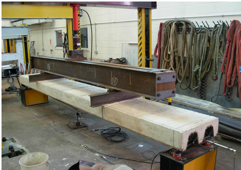
Figure 2: Test arrangement for composite slab tests
