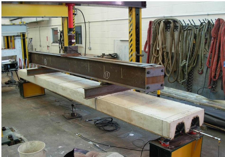
Figure 2: Test arrangement for composite slab tests
