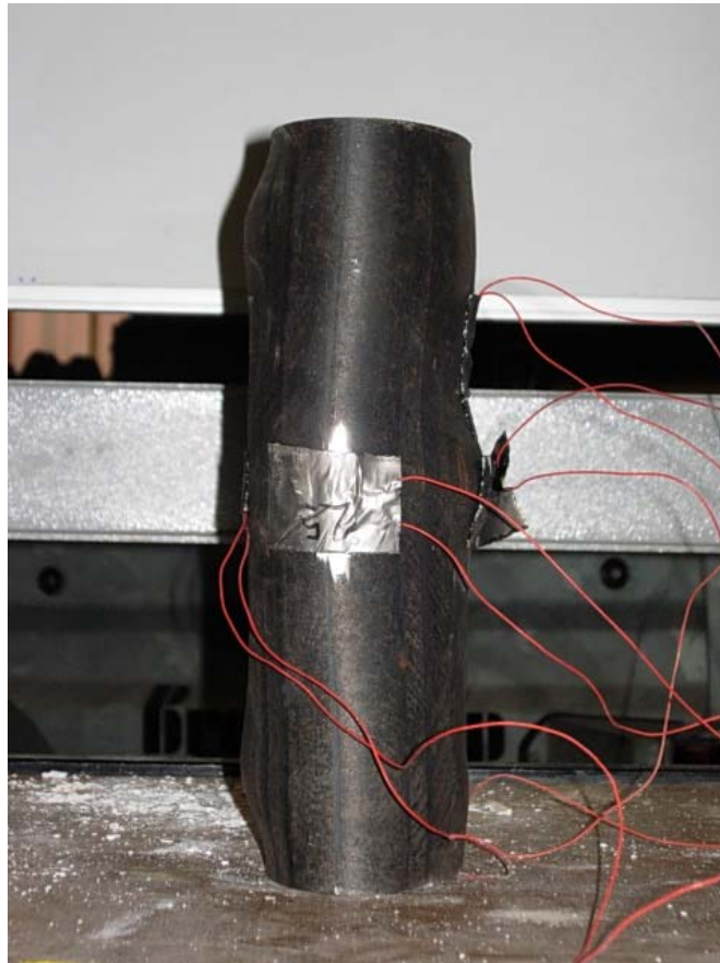
Figure 3: Typical failure mode of the composite EHS
