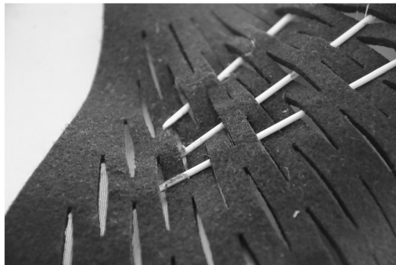
Fig. 2 Laser cut pattern on a synthetic felt allowing for shape-change
