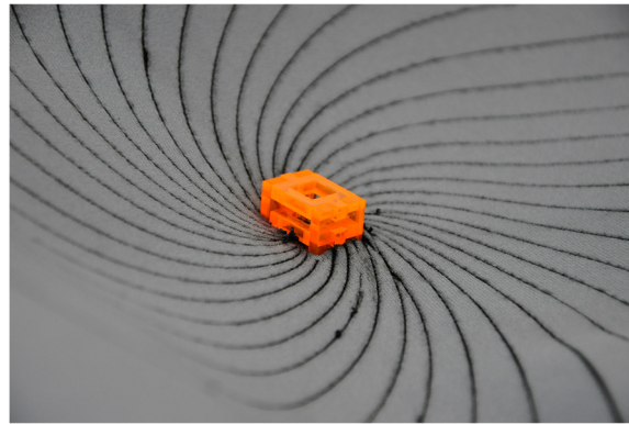
Fig. 3 Integration of vibration motors and 3D printed cases in an laser engraved neoprene textile
