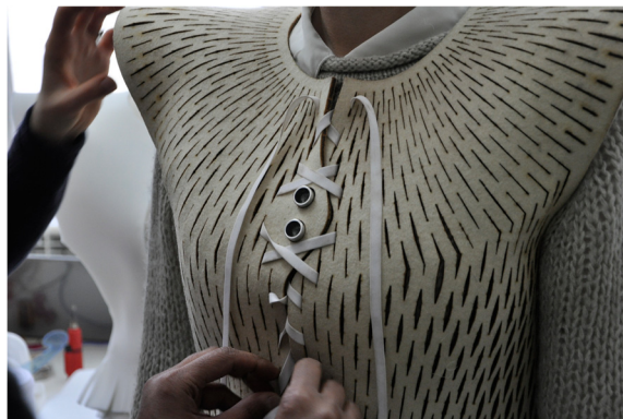
Fig. 5 Open Up (v.2) is made of proximity sensors and laser cut felt. It relates to the body by letting feel if something trespasses your ‘personal’ space. Its context of use is everyday life (e.g., walking on the streets)
