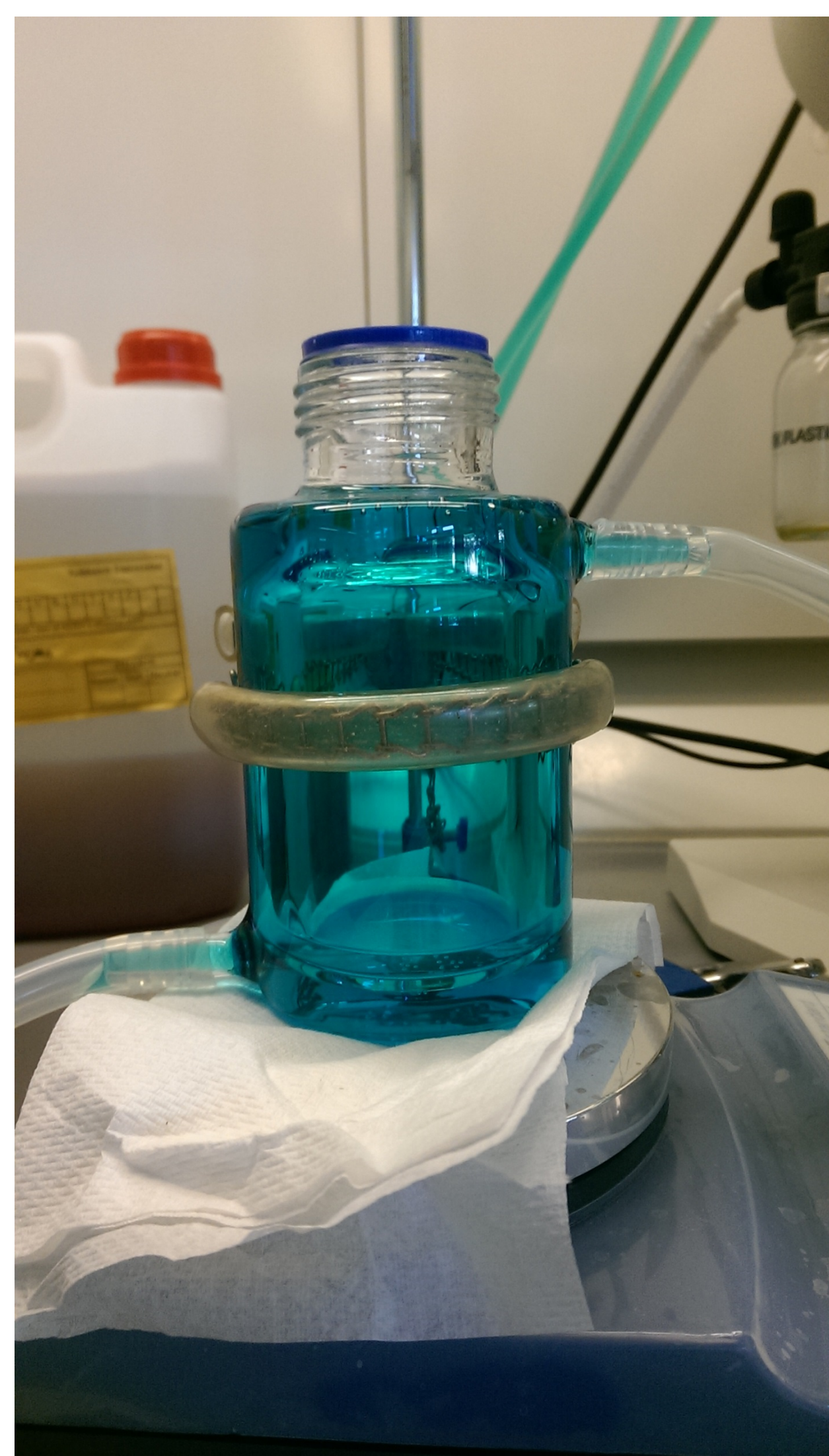
Glass reactor with 50/50 ethylene glycol/water cooling
