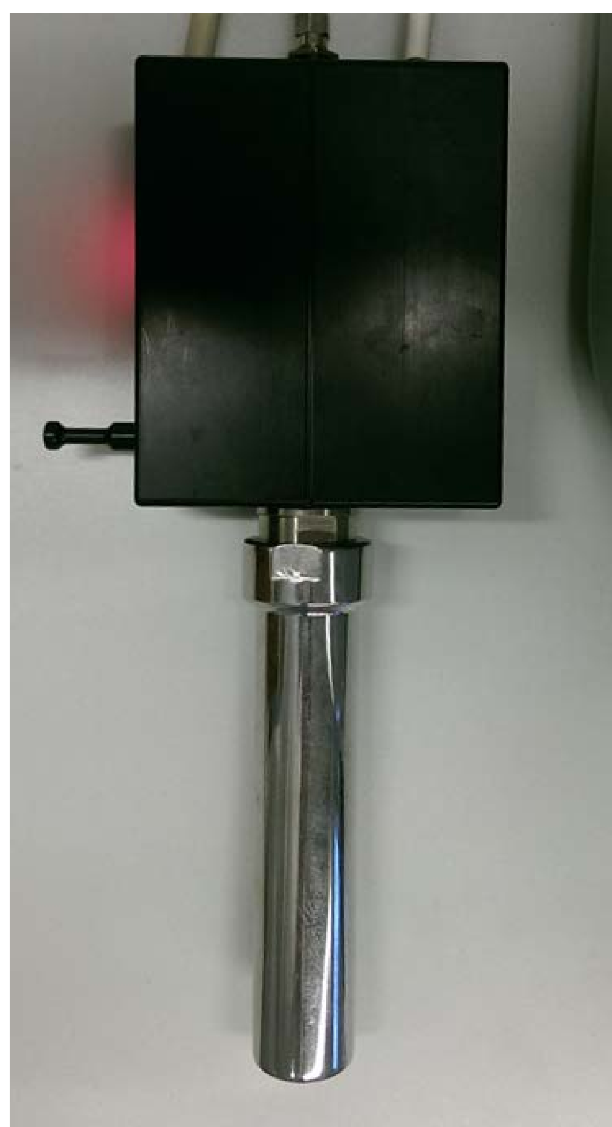
Raman probe and immersion tube
