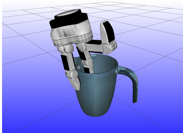
Fig. 15. Visualisation from RobWork showing a grasping action with the Schunk SDH-2 hand.
