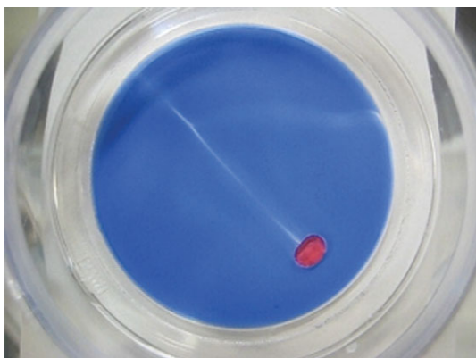
Figure 1. Droplet moving in an aqueous pool containing surfactant. Droplet (red) was moving from the upper left to the lower right edge. The low pH trail was visualized by using the pH-sensitive dye thymolphthalein. Diameter of the section containing the aqueous pool was 27 mm.
