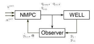
Figure 3: Float diagram
