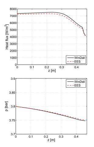
Figure 3: Comparison of the local heat flux and pressure in the channel for refrigerant R134a with uniform distribution of the airflow.
