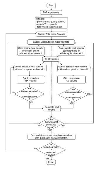
Figure 2: Flowchart of the model equations. The pressure drop and heat transfer calculations are performed inside the procedure HX\_volume.
