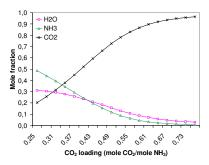
Figure 9: Composition of the bubble point gas phase of a 10wt% ammonia solvent with a temperature of  $110^{\circ}C$  as a function of the  $CO_2$  loading
