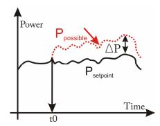
Figure 12: Delta production constraint
