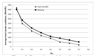
Figure 5 Comparing model results with experimental data ( $\Delta T_{w-g} = 18^{\circ}C$ , P = 1bar)
