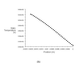
Figure 3: Predicted Temperature distribution in an x-y plane corner line along z direction. (a) ANSYS. (b) FLUENT.
