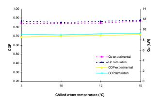
Figure 9: COP and cooling capacity (Qc) with an MGT output of 18 kW and an ambient temperature of 27 °C inside the environmental chamber.
