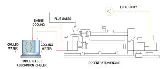
Figure 5. Schematic diagram of the ICE+SE trigeneration system
