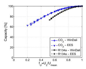
Figure 7: Comparison of the reduction of cooling capacity due to maldistribution of the airflow for R134a and CO<sub>2</sub> using both EES and WinDali.
