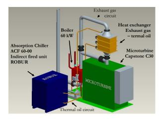
Figure 2: Main components of the trigeneration system
