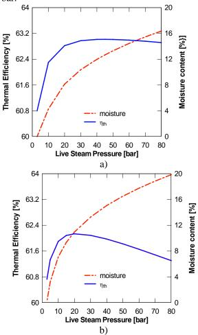
Figure 2. Thermal efficiency and moisture content of the combined SOFC – ST plants as function of live steam pressure, a) with CPO reformer, and b) with ASR reformer.
