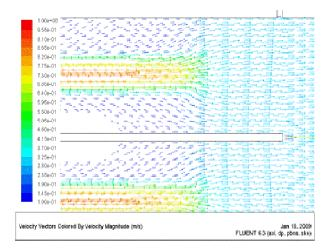
Figure 7: Contours of distribution of the Velocity vectors around the outlet of the lower channel
