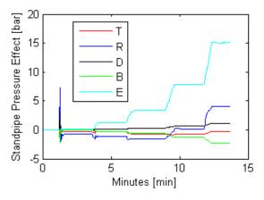
Figure 2 Main effects on standpipe pressure
