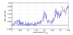
Figure 6: Variation of the max. Lyapunov exponent w.r.t the parameter  $T_{air,2}$ .
