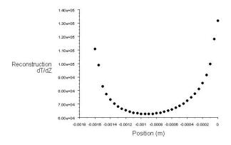
Figure 11: FLUENT 1D temperature gradient in an x-y plane corner line along z direction with convection.
