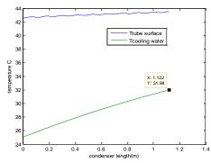
Figure 6. Distribution of the wall and the fluid temperatures for the condenser
