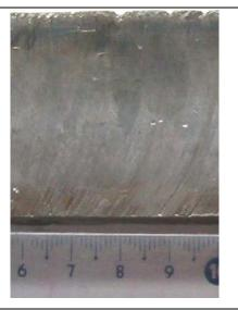
Fig.11. Cut surface of the lead plate with 45 mm thickness
