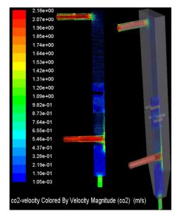
Figure 9 Velocity Profile inside the condenser model
