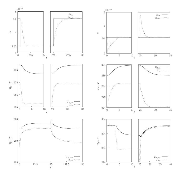
Figure 3:  $\dot{m}$ ,  $T_W$ , and T at z=0 (in) and z=10 m (out) as a function of time when the inlet massflow  $\dot{m}_{in}$  is reduced by a factor of two at t=0.5 s and increased again to the initial value ( $5.3 \cdot 10^{-3}$  kg/s) at t=25 s. Time axis is broken in upper and middle plot to exclude the non-varying part of the functions. Units refer to Table 1.
