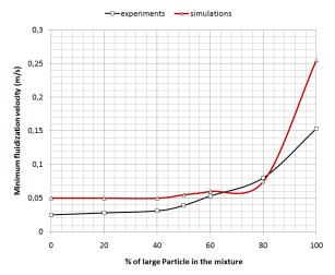
Figure. 3 Experimental and computational minimum fluidization
