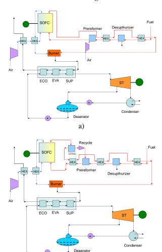
Figure 3. Combined SOFC – ST cycle plants with cathode preheating in the SOFC cycle, a) with CPO reformer, and b) with ASR reformer.
