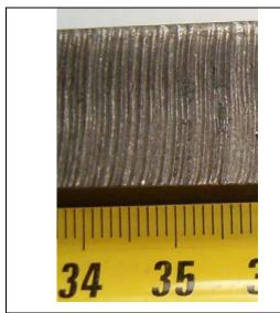
Fig.10. Cut surface of the S 335 J2 steel plate with 20 mm thickness
