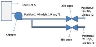
From data-base: 40 m3/h - 17 + 25 m3/h - no balanceBalance calculation with model gives: 39 m3/h = 17.5 + 21.5 m3/h,
