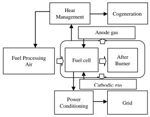
Figure 2 Micro CHP system configuration
