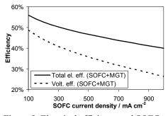
Figure 5: Electrical efficiency and SOFC voltage efficiency as a function of SOFC current density
