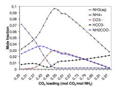
Figure 5: Composition of the liquid phase of a 10wt% ammonia solvent with a temperature of 8°C as a function of the CO<sub>2</sub> loading
