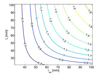
Figure 4: Contours of the mean flux density as a function of external radius and length. Each contour is labeled by its mean flux density. The maximum flux density is obtained by maximizing both  $r_{\rm ex}$  and L.
