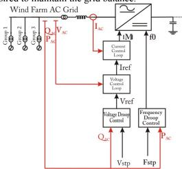
Figure 10: Block diagram of the WF Side Converter Controller
