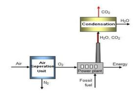
Figure 1 schematically representation of oxy-fuel process
