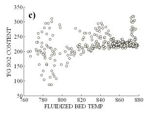
Figure 2: Emission models after creating a 24\*16 SOM. a) NO<sub>x</sub>, b) CO and c) SO<sub>2</sub> content [mg/Nm<sup>3</sup>] of flue gas (FG) as a function of the bed temperature [°C] by using the reference vectors of SOM neurons.
