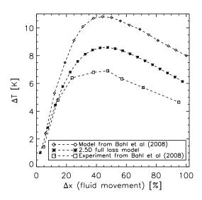
Figure 10: An example of the impact of including the thermal parasitic losses (denoted 2.5D full loss model). The losses are seen to have a significant impact on the experimental results. Reproduced from [12].
