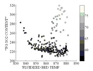
Figure 6: Flue gas (FG) SO<sub>2</sub> content [mg/Nm³] as a function of the bed temperature [°C] by using the reference vectors of SOM neurons in the process state of high steam flow. Color scale indicates the deviation of the furnace middle level temperature [°C].
