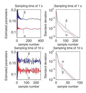
Figure 4: Effects of different sampling times on the slow fouling data series. Right: Estimated values of  $\alpha$  and  $\beta$ . Left: Evolution of the standard deviation.
