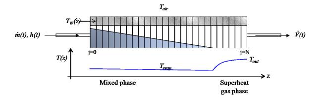
Figure 1: Schematic of evaporator model and dependent variables and parameters.
