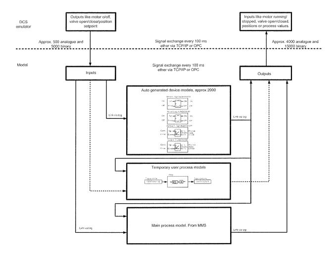
model and emulator but now it has been setup as a training station. The resemblance in topology of the hardware and software (DCS and models) that goes into simulating during phase two and the phase three is high.
