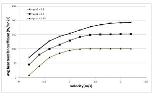
Figure 7 Average heat transfer coefficient as a function of inlet velocity and CO<sub>2</sub> mass fraction
