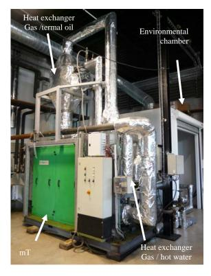
Figure 3: Trigeneration system in the CREVER-URV test bench
