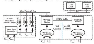
Figure 3: Control structure of the Wind Power System
