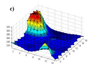
Figure 4: The component planes of different emission components  $[mg/Nm^3]$ , a)  $NO_x$ , b) CO and c)  $SO_2$ , on 18\*14 SOM grids after modeling the process state of **high steam flow**.
