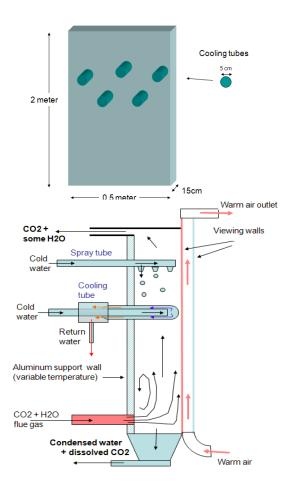
Figure 2 Proposed geometry for condensation study
