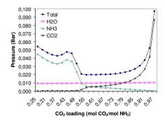
Figure 7: Bubble point pressures of a 10wt% ammonia solvent with a temperature of 8°C as a function of the CO<sub>2</sub> loading
