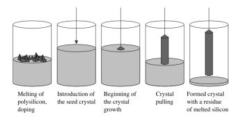
Figure 1: The Czochralski process, principle of operation. Illustration from Wikipedia.
