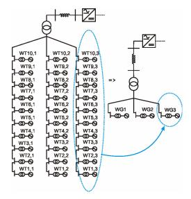
Figure 6: Multi-machine equivalent
