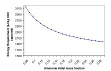
Figure 11: Energy requirement as a function of the initial mass fraction of ammonia, at a constant rich CO<sub>2</sub> loading of 0.67
