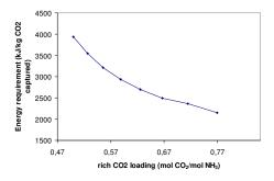
Figure 10: Energy requirement as a function of the loading of the CO<sub>2</sub>-rich stream, at an initial mass fraction of 10% ammonia
