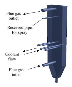
Figure 3 First implemented model for condenser
