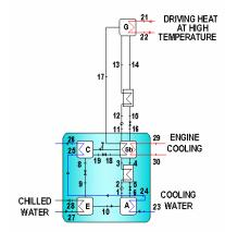
Figure 2. Schematic diagram of a DE absorption chiller
