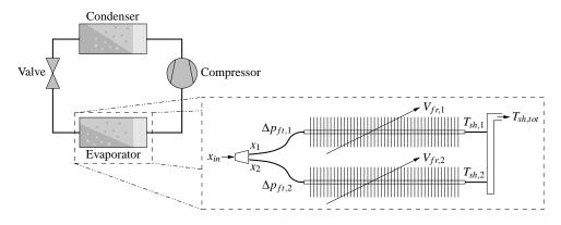
Figure 1: Sketch of model setup
