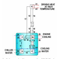
Figure 3. Schematic diagram of a SE/DE absorption chiller
