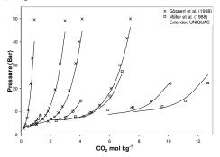
Figure 3: Total pressure in NH<sub>3</sub>-CO<sub>2</sub>-H<sub>2</sub>O mixtures at 120°C
