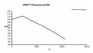
Figure 10: Pressure profile of pipeline CR0TT with design flow rates, open outlet to MF-T11.
