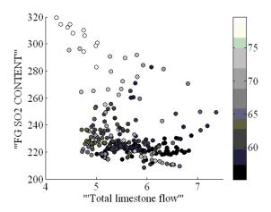
Figure 7: Flue gas (FG) SO<sub>2</sub> content [mg/Nm<sup>3</sup>] as a function of the limestone flow [kg/s] by using the reference vectors of SOM neurons in the process state of high steam flow. Color scale indicates the deviation of the furnace middle level temperature [°C].
