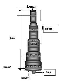
Figure 1. The pulping digester.
