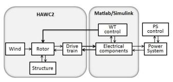
Figure 1: Wind power integrated design platform: HAWC2 - Matlab
