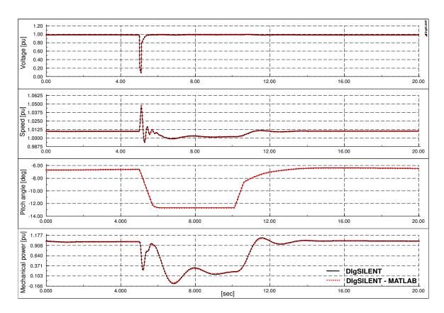
Figure 8: Simulation comparison between the benchmark model inside DIgSILENT and the proposed online simulation approach between MATLAB and DIgSILENT.
