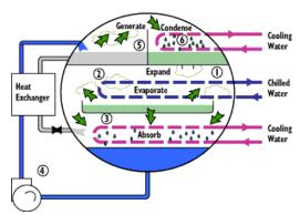
Figure 1. absorption machine
