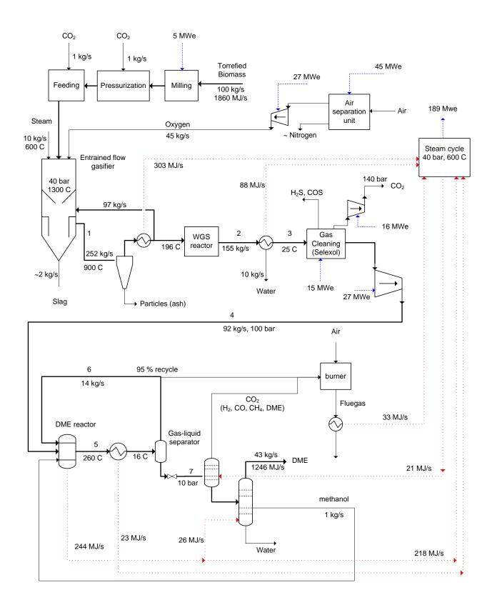
Figure 1. Flow sheet of the modeled DME plant. Some important parameter values are shown.
