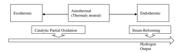
Figure 5 Hydrogen output as function of operating conditions
