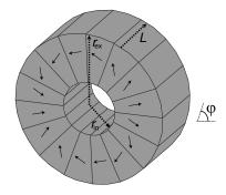
Figure 3: A illustration of a 16 segmented Halbach magnet. Shown as arrows is the direction of magnetization. The internal and external radii,  $r_{in}$  and  $r_{ex}$ , respectively, and the length, L are also shown.
