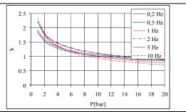
Fig.2. Polytropic factor at dynamic HRG gas compression cycles with frequencies between 0.2 Hz and 10 Hz
