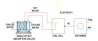
Figure 6. Schematic diagram of the FC+SE trigeneration system
