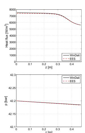
Figure 4: Comparison of the local heat flux and pressure in the channel for refrigerant CO<sub>2</sub> with uniform distribution of the airflow.
