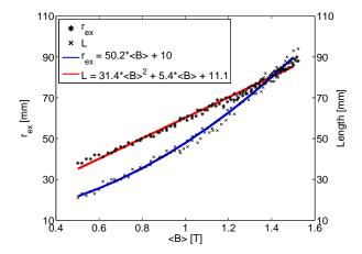
Figure 6: The optimal  $r_{\rm ex}$  and L as functions of the mean flux density. Polynomia have been fitted to the data to ease interpolation. Building a Halbach cylinder with an internal radius of 21 mm with dimensions different from the dimensions given here means that more magnetic material is used than need be, if one does not care about the volume of the bore.
