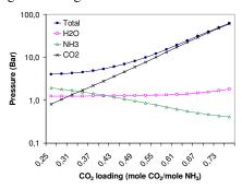
Figure 8: Bubble point pressures of a 10wt% ammonia solvent with a temperature of 110°C as a function of the CO<sub>2</sub> loading
