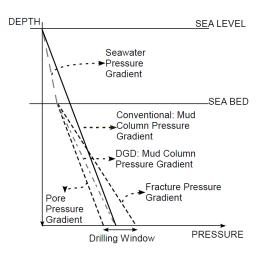
Figure 1: Hydrostatic pressure profile for dual gradient and conventional drilling
