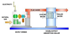
Figure 7. Schematic diagram of a MGT+DE trigeneration system
