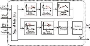
Figure 9: WF Controller block diagram
