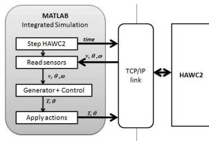
Figure 4: Integrated simulation simplified flow diagram
