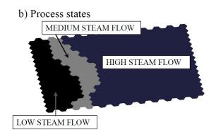
Figure 3: a) The behavior of the main steam flow on a 24\*16 SOM, and b) Clustered SOM (k = 3), which shows the separation of process states into three categories.
