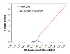
Figure 6: Nature and amount of solid phases of a 10wt% ammonia solvent with a temperature of 8°C as a function of the CO<sub>2</sub> loading
