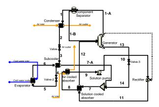
Figure 8: Flowsheet of the absorption chiller model in Aspen Plus
