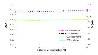
Figure 10: COP and cooling capacity (Qc) with MGT output of 20 kW and air temperature at 28 °C inside the environmental chamber.
