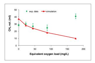
Figure 5: Experimentally determined (average±SD) and simulation predicted ultimate methane generation vs. oxygen load
