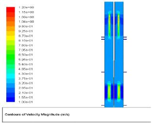
Figure 4: Contours of distribution of the Velocity in the two formed channels
