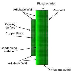
Figure 4 Illustration of solution domain and boundary condition
