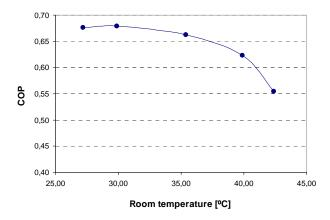
Figure 4: COP of the absorption chiller as a function of ambient temperature for an electrical output power of 20 kW, a chiller temperature of  $8^{\circ}$ C and a thermal oil flow rate of  $2400 \, l/h$
