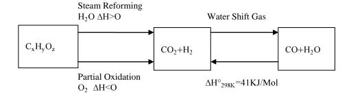
Figure 6 Flow diagram of different combination of reforming reactions
