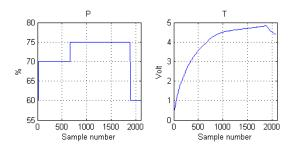
Figure 2: Timeseries *P* and *T* used for identification of the transfer function from *P* to *T*.
