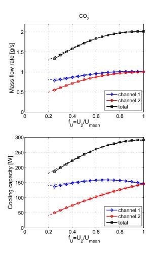
Figure 6: Influence of airflow maldistribution on the mass flow rate and cooling capacity of the two channels using  $CO_2$  as refrigerant. The solid lines with markers shows the results obtained using WinDali, and the dashed lines show the results using EES.
