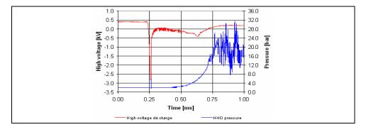
Fig. 5. Electrical discharge high voltage and pressure-time history at HRG gas burning
