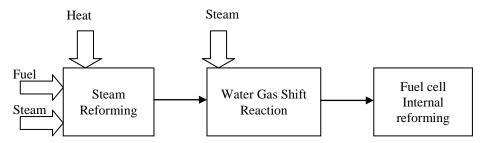
Figure 3 Fuel reforming process
