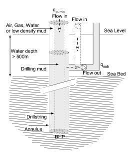
Figure 2: Dual-Gradient Drilling flow schematic
