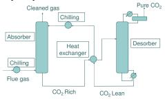
Figure 1: Flow sheet of the process
