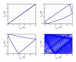
Figure 3: Typical limiting behaviors with the various values of the parameter  $T_{air,2}$ . (a) 2-periodic limit cycle (synchronization,  $\overline{T_{air,2}} = 0$ ), (b) 4-periodic limit cycle ( $T_{air,2} = 0.1\overline{5}$ ), (c) another 4-periodic limit cycle ( $\overline{T_{air,2}} = 0.2$ ), (d) high-periodic limit cycle ( $T_{air,2} = 0.3$ ).
