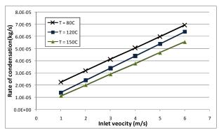
Figure 8 Condensation rate as a function of inlet velocity and inlet temperature
