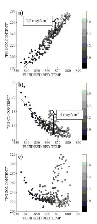
Figure 5: Emission models of the process state of **high steam flow**. a) NO<sub>x</sub>, b) CO and c) SO<sub>2</sub> content [mg/Nm<sup>3</sup>] of flue gas (FG) as a function of the bed temperature [°C] by using the reference vectors of SOM neurons. Color scale indicates the deviation of the bed temperature [°C].
