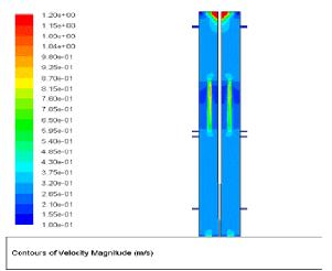
Figure 3: Contours of distribution of the Velocity at the top of the digester
