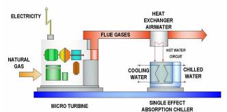
Figure 4. Schematic diagram of the MGT+SE trigeneration system
