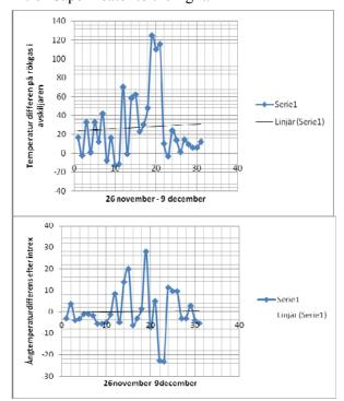
**Figure 6.** The deviation between calculated and measured temperature in the separator ("cyclone") to the left and in the Intrex Super Heater steam temperature during a two week period to the right.
