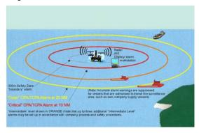
Figure 8: Alarm boundaries for a typical floating production system.
