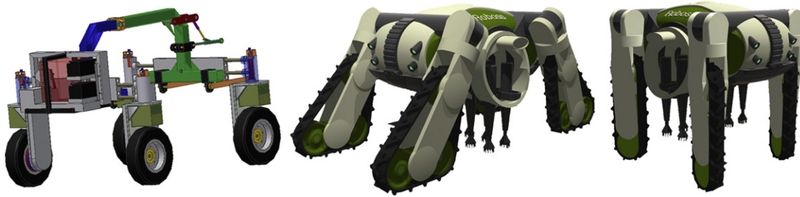
Fig. 4 – Examples of two conceptual designs of a future plant nursing robot. Left: the engineering approach HortiBot II by Petersen et al. (2006). Right: the industrial design approach Roboss by Sørensen, 2006.
