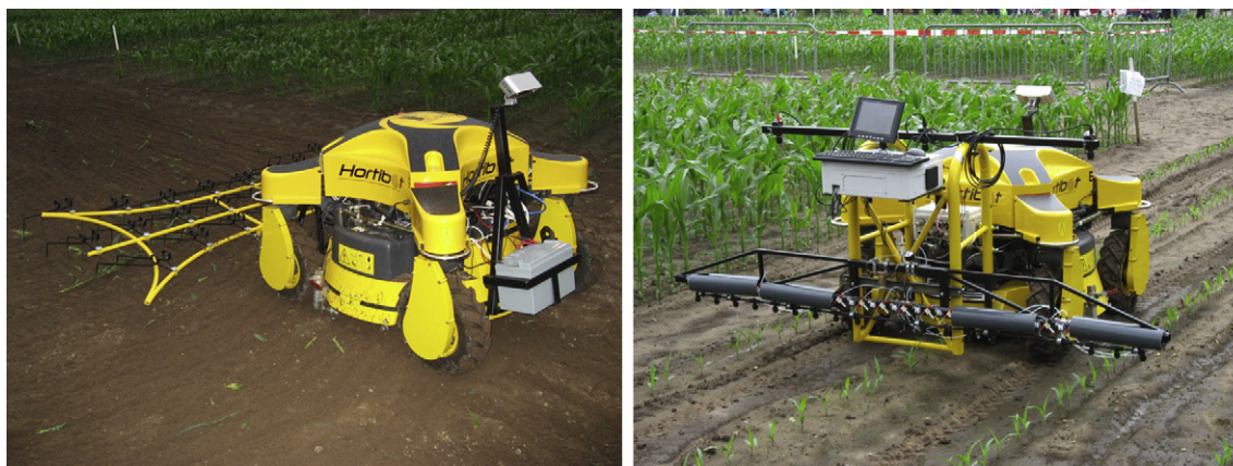
Fig. 1 – The small plant nursing robot, HortiBot, with two different weeding tools: a herbicide cell sprayer and a tyne weeder. The system was presented at the annual Field Robot Event 2007 in Wageningen in the Netherlands.
