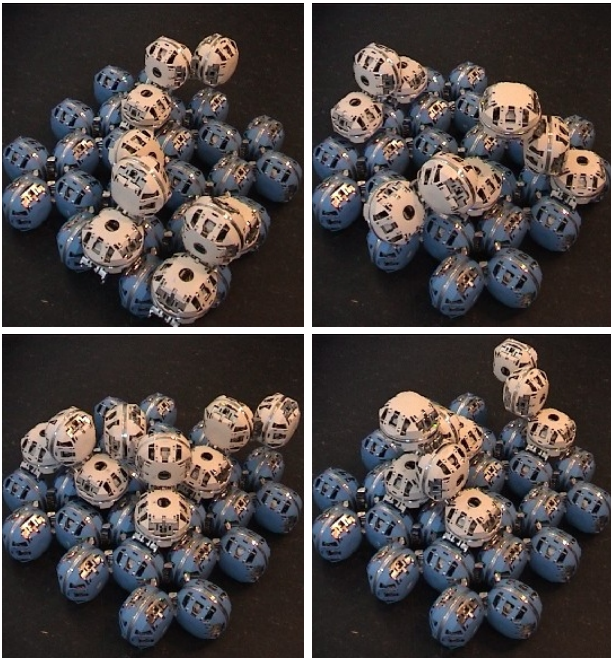
Fig. 7. In this trial three meta-modules move on the same surface of modules. They do not communicate so they collide with one another, but the control system is able to tolerate this so that they can co-exist.
