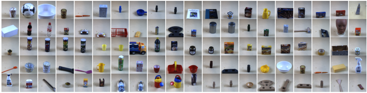
Fig. 8. Multi-view dataset of 100 objects shown in thumbnails. The set contains RGBD and stereo images: 30 samples each object from three camera views. The data were captured under three lighting conditions. The dataset is available at http://caro.sdu.dk/sdu-dataset (we will make it available by the final submission of this manuscript).
