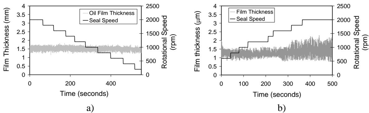
Figure 14. Plots of (a) oil film and (b) water film thickness variation with time as seal rotational speed is varied. Constant sealed fluid pressure of 10 bar.
