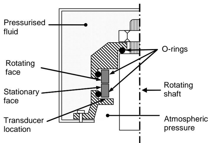
Figure 11. Schematic diagram of mechanical face seal
