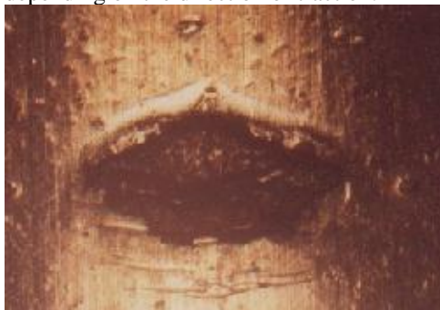
Figure 10. A fatigue spall initiated at a debris dent on a rolling bearing raceway.
