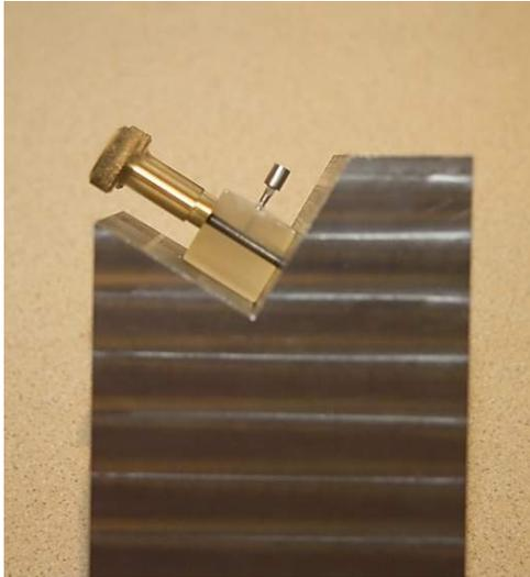
Fig1: Each implant/crown assembly was mounted in an acrylic block which was itself secured in the cradle of the steel mounting block. This set-up held each implant with axis off-set 30° from the vertical (as per ISO 14801; 2003).
