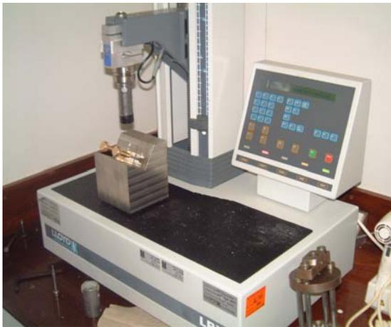
Fig 2: Mounted samples on the steel block were positioned under the vertical ram of the Tensometer (Lloyds Instruments Ltd, Hants, UK). With the ram traveling at 1mm/Min, continuous output data recorded the load applied and distance traveled by the ram.
