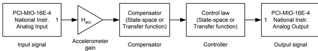
**Figure 7: A basic Simulink model of controller**
