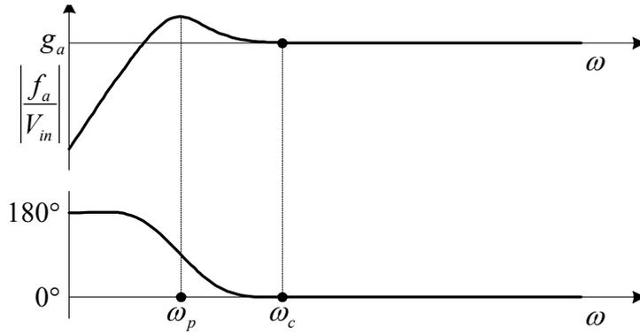
Figure 2: Bode plot of an idea proof-mass actuator
