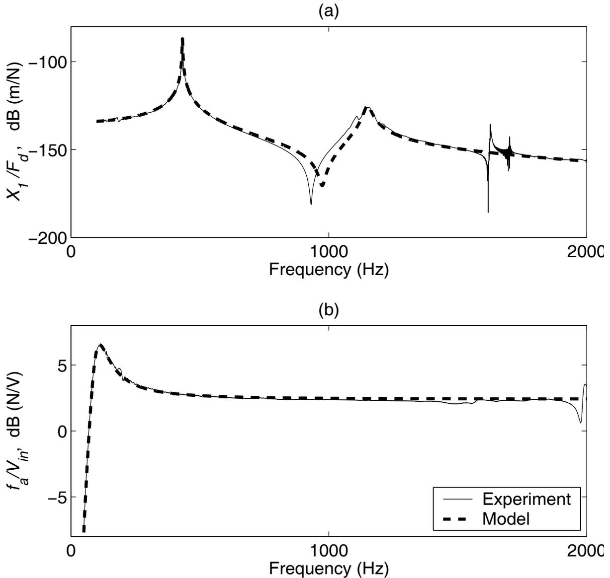
**Figure 6: Experimental and modelled frequency response functions.**
