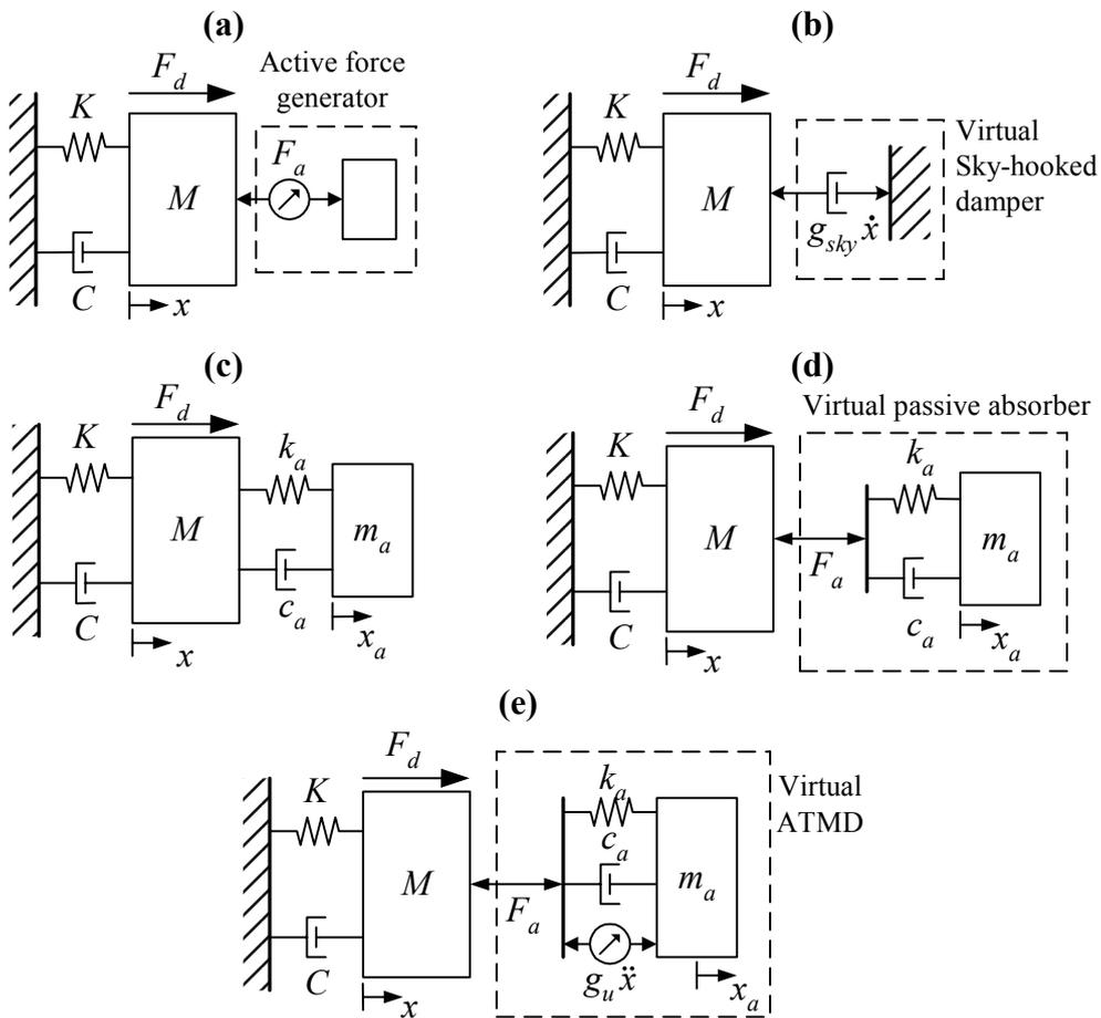
Figure 3: Schematic representation of the control laws. (a) Proof mass actuator performing active vibration control (b) Virtual skyhook damper (c) Passive vibration absorber (d) Virtual passive absorber (e) Virtual active tuned mass damper, or virtual passive/active absorber
