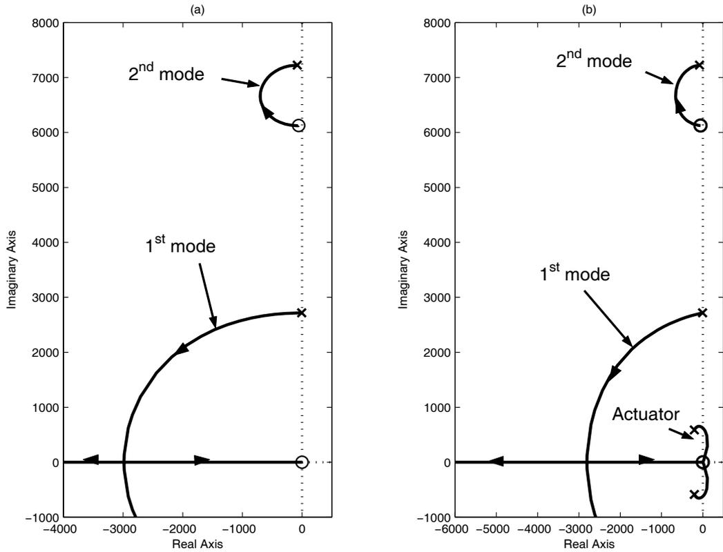
**Figure 8: Root-locus plot of the structure with virtual skyhook damping.**
