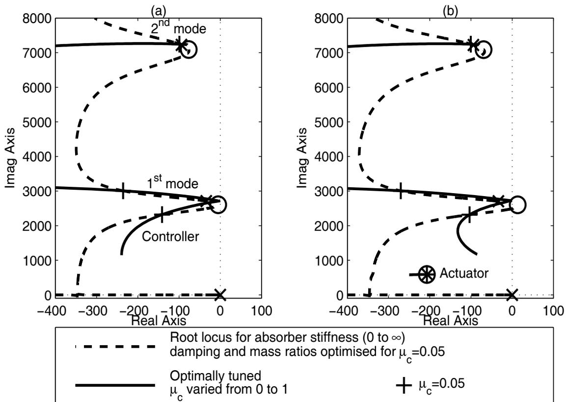
**Figure 9: Loci of characteristic roots of the structure with virtual passive absorber controller.**
