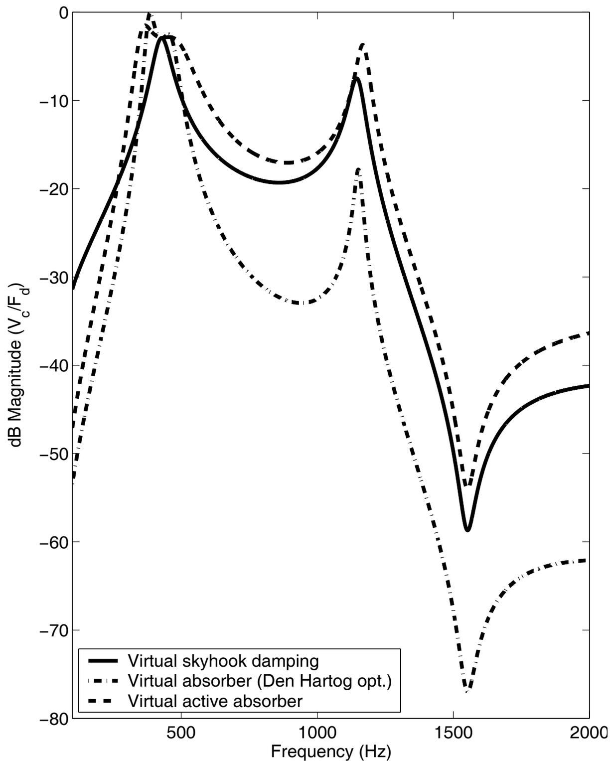
Figure 12: FRF of the control voltage as a function of disturbance force.
