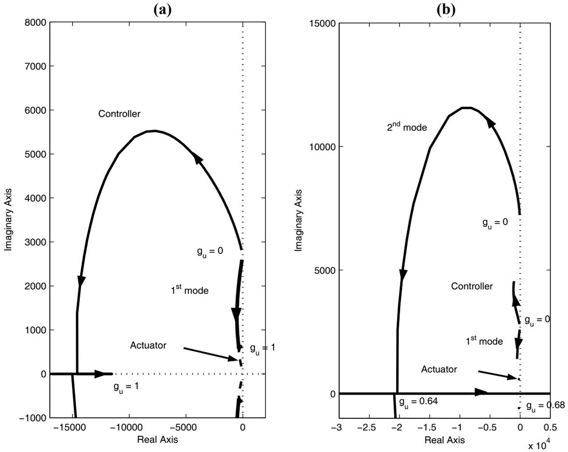
Figure 10: Loci of characteristic roots of the structure with virtual passive/active absorber controller with actuator dynamics. (a) 1DOF structural model (b) 2DOF structural model
