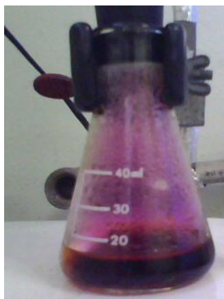
Figure 3. Formation of elementary iodine crystals and also \text{I}_2 gas
