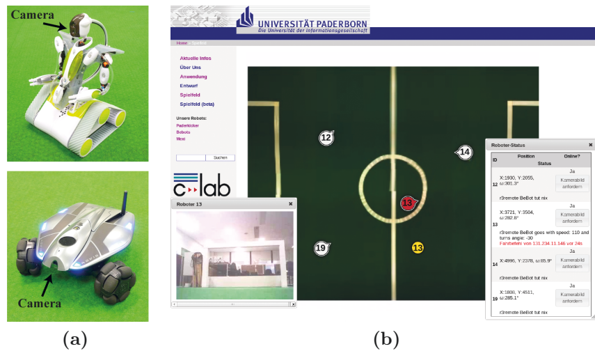
Figure 5.14: (a) Commercial robotic platforms that were integrated into the test bed. (b) Web-client of the test bed.
