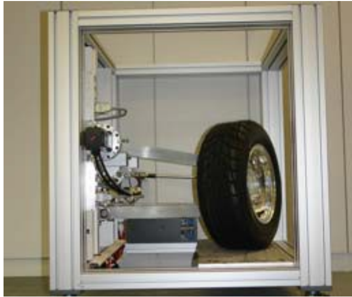
Figure 8.4: Wheel and damping testbed
