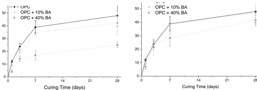
Figure 3. The Effect of OPC replacement by BA on Strength Development. (The figure on the right shows the strength normalised to the cement content)
