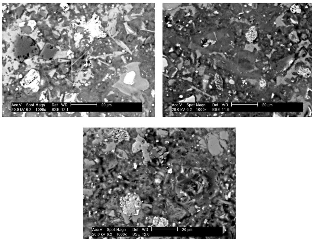
Figure 1. SEM of (a)OPC (b)OPC+10%BA (c)OPC+40%BA
