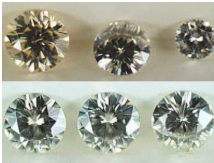
Figure 1.2: The upper picture shows three moissanite crystals (0.12 ct) in nearly colorless till light yellowish. The bottom picture shows (from left to right) a synthetic moissanite, a brilliant, and a synthetic zirconia.[1]
