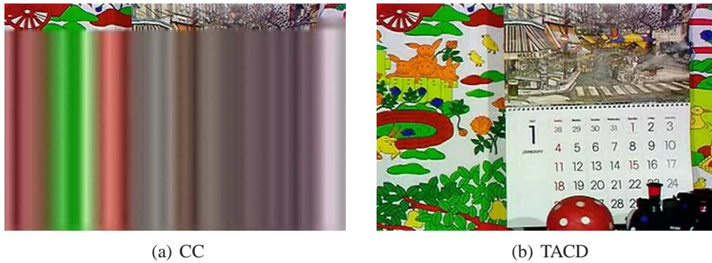
Figure 5.6: Frame 1 of the MAF video sequence; received at equal instantaneous SNR using CC or TACD.
