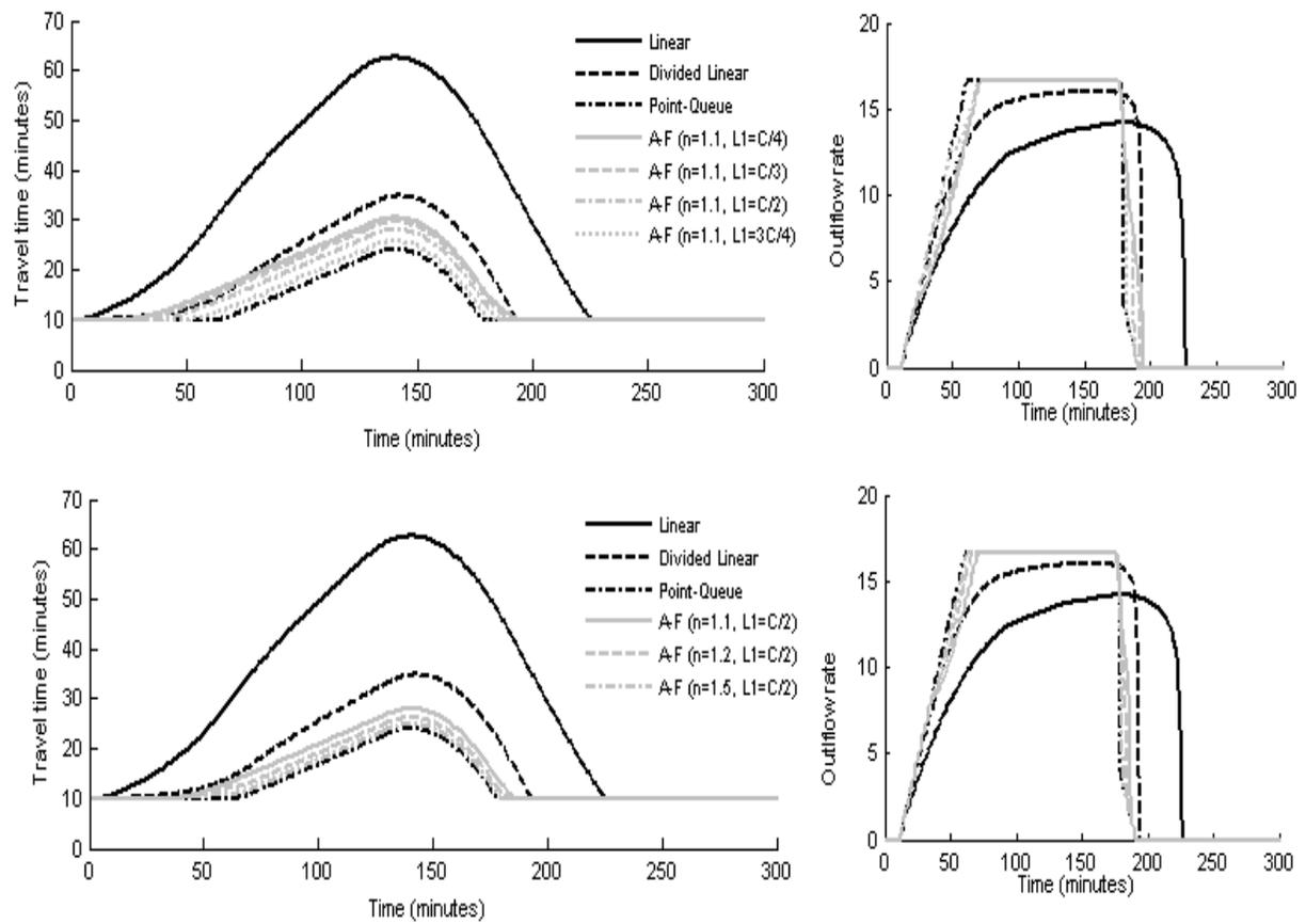
**Figure 8:** 3<sup>rd</sup> Case Travel time and Outflow Profiles for dynamic loading models
