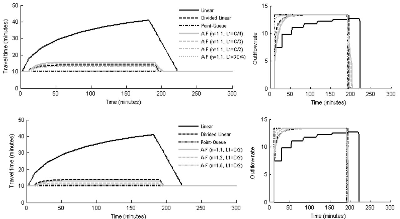
**Figure 4:** 1<sup>st</sup> Case Travel time and Outflow Profiles for dynamic loading Models
