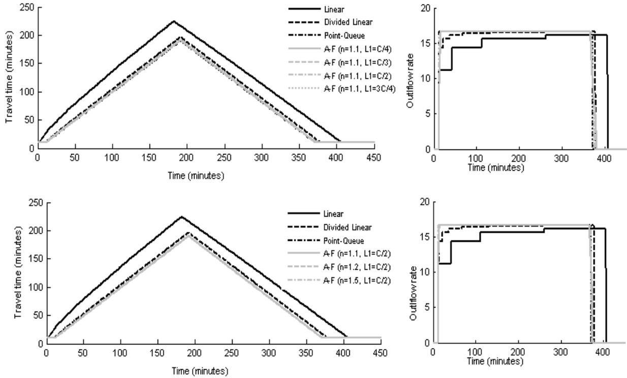
**Figure 6:** 2<sup>nd</sup> Case Travel time and Outflow Profiles for dynamic loading models
