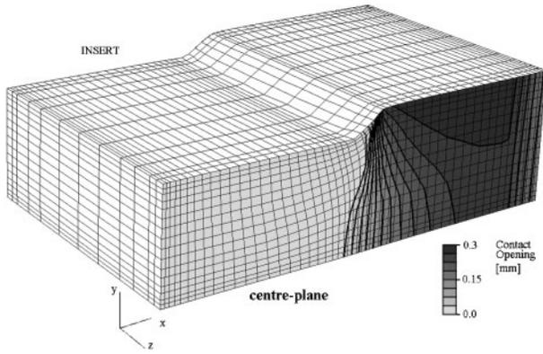
**9 Contact opening between workpiece and insert on centre plane**
