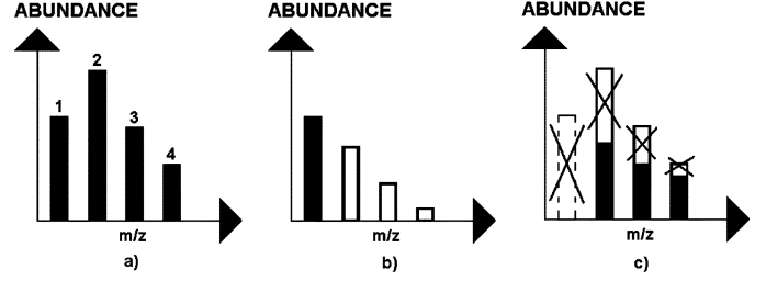
Fig. 1. Deisotoping example. (a) Overlapped peaks. (b) Isotopes of peak 1. (c) Deisotoped residuals.
