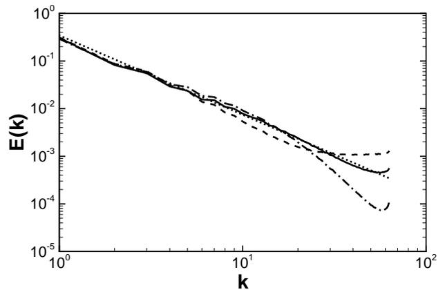
FIG. 3: Radial kinetic energy spectra of forced isotropic turbulence from LES using the matrix-exponential closure of Eq. 19 with  $c_{\text{exp}} = (0.1)^2$ . Solid line:  $\gamma = 1$ , dash-dotted line:  $\gamma = 2$ , and dashed line:  $\gamma = 0.5$ . Dotted line: universal Kolmogorov spectrum  $E(k) = 1.6\epsilon_f^{2/3}k^{-5/3}$ .
