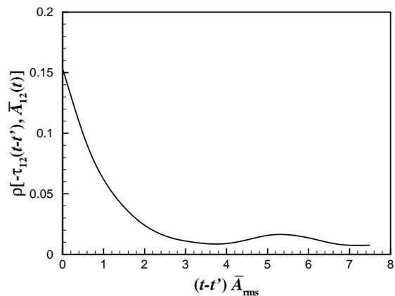
FIG. 2: Decay of the correlation coefficient  $\rho$  (see Eq. 12) between  $\tau_{12}(t - t')$  and  $-\overline{A}_{12}(t)$  as function of normalized time lag  $(t - t')\overline{A}_{\text{rms}}$  measured in DNS of isotropic turbulence.
