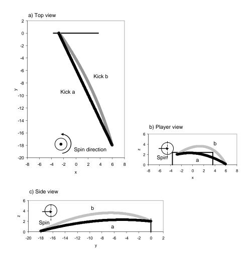
Figure 9. Predictions for the flight of two curving free kicks based on type of ball.
