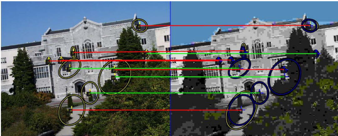
FIG. 5.72: An example of nearest-neighbor matching using SIFT-Based-SSC descriptor computed for Harris-Affine regions. The results are obtained for the structured scene, ubc of Fig. 5.2h. The detected regions are in yellow while their correspondences transformed from the reference (image in the left of each sub figure) to the second (image in the right of each sub figure) using ground truth are in blue. The region correspondences computed based on ground truths and overlap errors are highlighted with blue lines whereas matches identified as correct using descriptors are highlighted with green lines. For the purpose of clarity, only few correspondences are shown.
