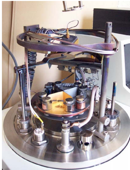
Figure 3.1: Evaporator chamber used in ohmic contact fabrication.
