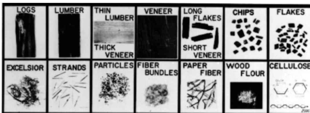
Fig. 3.7: Basic wood elements (largest → smallest) [52]
