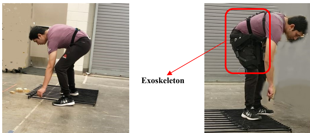
Fig. 4: Performing simulated rebar task: (a) NoExo condition; (b) Exo condition.
