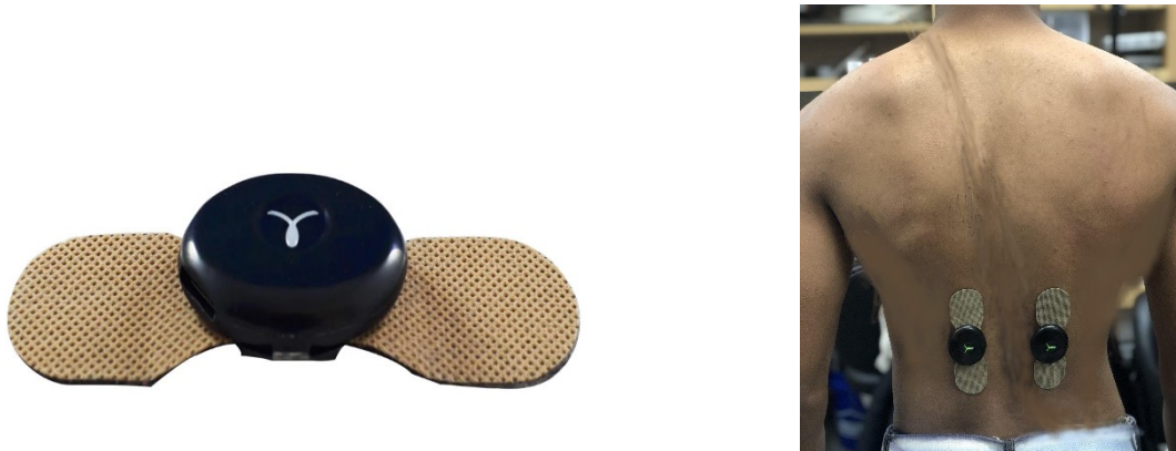
Fig 3: (a) Cricket wearable device (left); (b) Cricket devices on the left and right erector spinae muscles (right).
