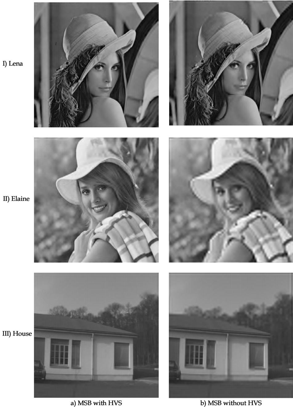
Fig. 10. Reconstructed I) 'Lena', II) 'Elaine' and II) 'House' test images at compression ratio of 16 using the MSB codec a) with HVS and b) without HVS.
