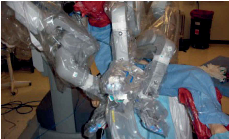
Fig. 3. The da Vinci® Si HD system side-docked with intersected robotic arms and the patient in a modified lithotomy position; the left leg is slightly extended and the hip abducted (low lithotomy), whereas the right leg is flexed at the level of the knee and hip (high lithotomy)
