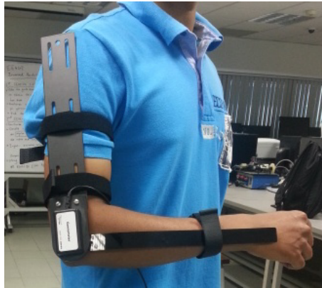
Figure 5.15: Angle measurement setup using electronic goniometer
