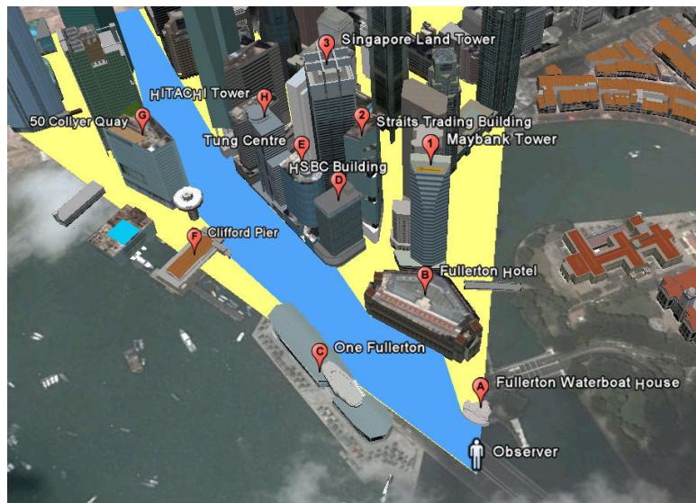
Figure 3.2: Illustration of a sample FOVScene and the visible objects which are supplied by Google Earth and determined by conducting geometry computations (Copyright © 2013 Google).
