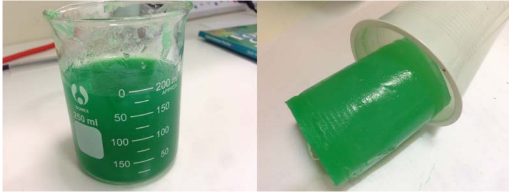
Figure 5.2 Condition of the agar-based mixture: liquid when heated to greater than 50° Centigrade (left); solid at room temperature (26° Centigrade, right).
