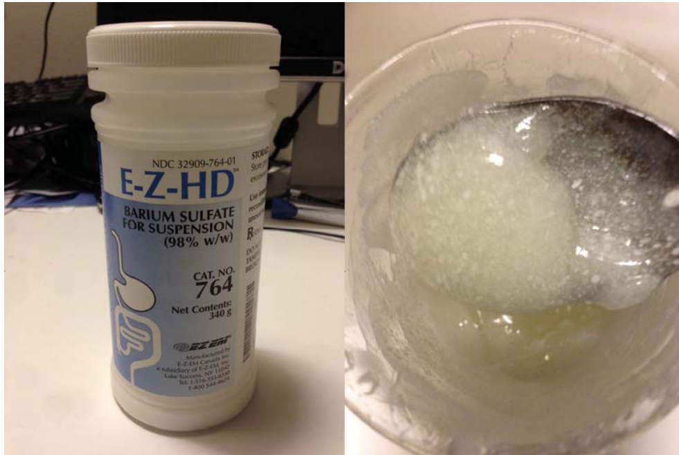
Figure 5.4 Addition of clinical barium sulfate to the Vaseline-based mixture
