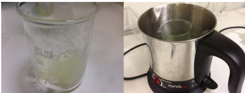
Figure 5.3 Making the Vaseline-based tumor model: Vaseline jelly (left); hot water bath (right).
