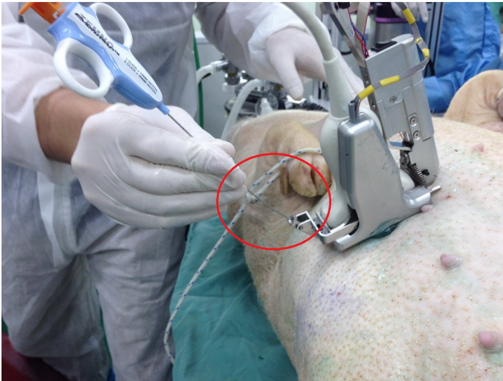
Figure 5.9 Biopsy attempt without cutting the abdominal skin of the micropig. The red circle shows the bending of the biopsy needle during insertion
