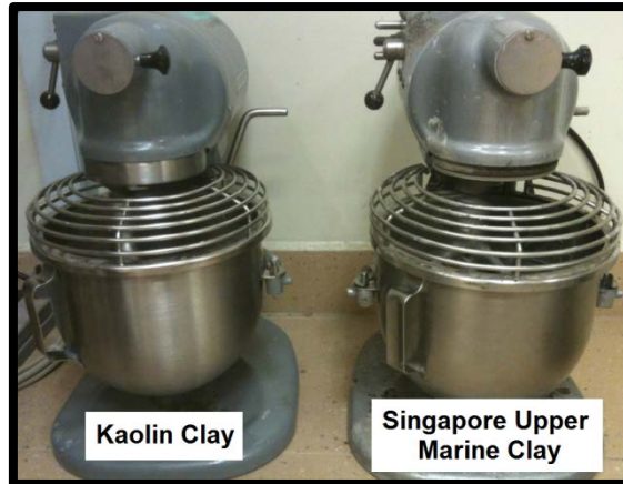
Figure 3.3 Mixing of Kaolin Clay and Upper Marine Clay slurries.
