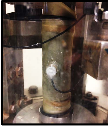
Figure 3.10 Mid-plane pore pressure transducer in resonant column setup.
