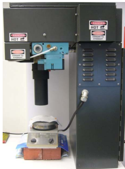
Fig. 2-1 Collimated beam apparatus for UV disinfection
