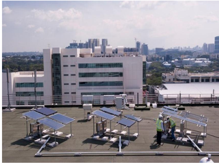
Figure 3.2: Outdoor PV module performance testing system at NUS.
