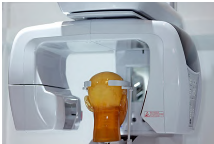
Figure 2.6: Cone-beam computed tomography system. A phantom is stabilized with a head holder (from U.S. Food and Drug Administration website).
