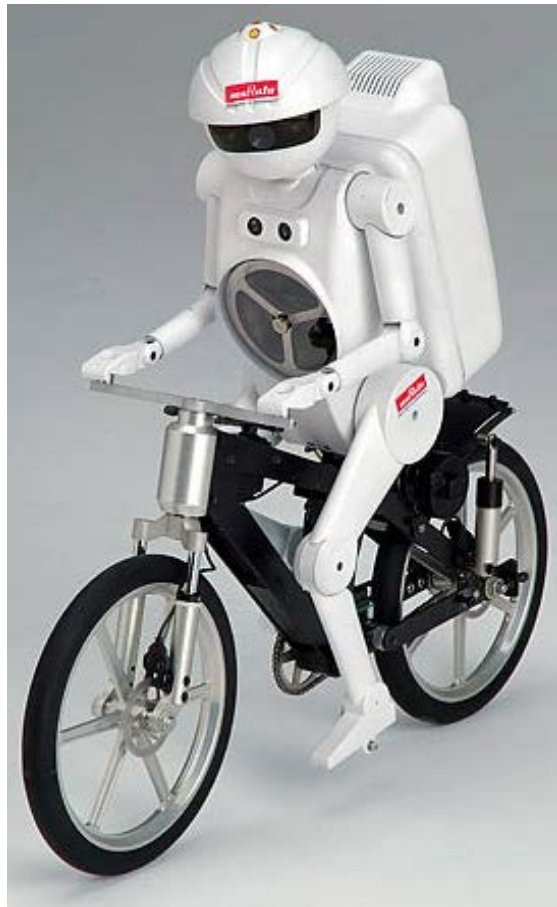
Figure 1.1: Murata Boy [10], self-balancing riding robot.
