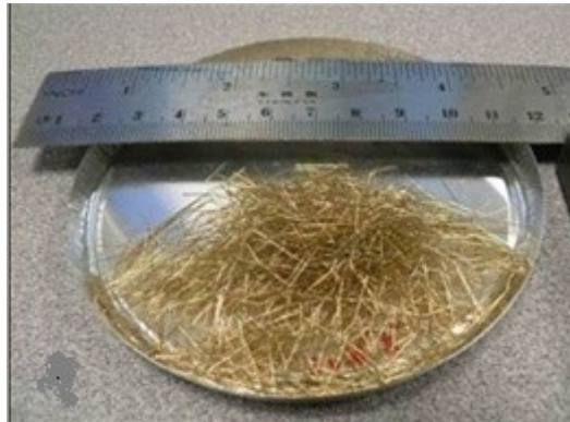
Figure 4.1: High tensile strength steel fiber - SF 13/80
