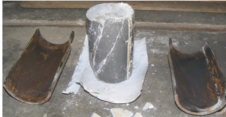
(a) S1-2-1(a) loaded only on UHSC core
