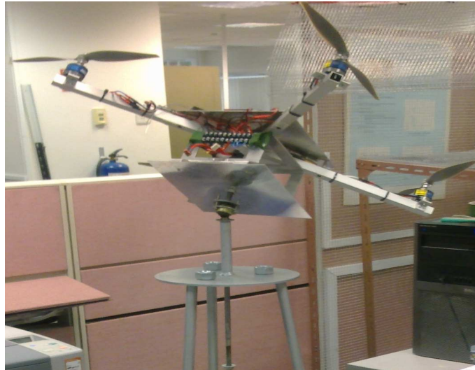
Figure 2.1: First developed quadrotor body, mounted on the regulator stand.
