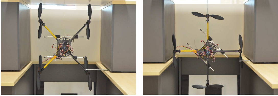
Figure 3.5: Finding the CG location. Left: Captured picture. Right: Printed intersectional lines.
