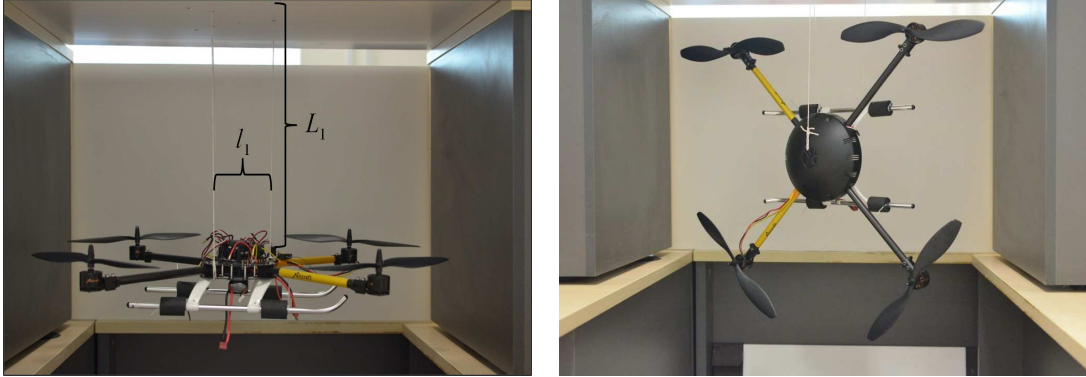
Figure 3.4: Left: J_{zz} measurement experiment setup. Right: J_{xx}, J_{yy} measurement experiment setup.
