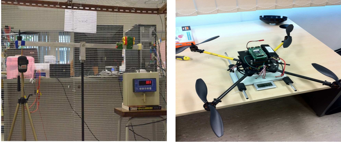
Figure 3.3: Left: rotor thrust measurement stand. Right: measuring the whole platform weight.
