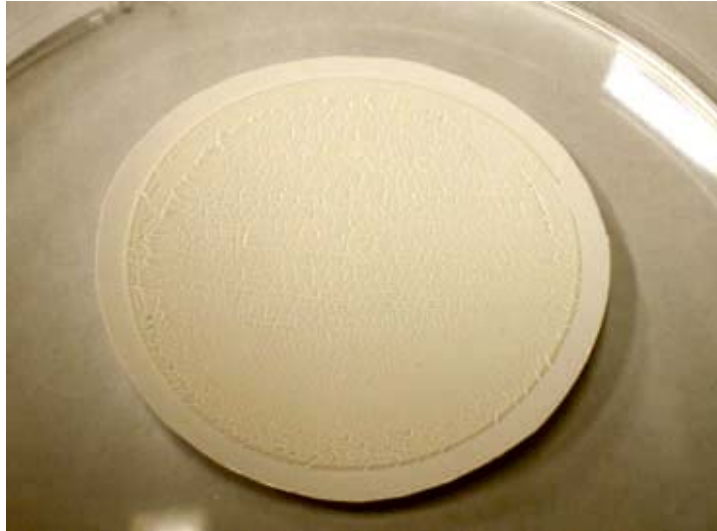
Figure 6.11 Photograph of air-dried fouled membrane after two hours of filtration with 1000 ppm P4VP250. Note the thick cake layer on the membrane surface.
