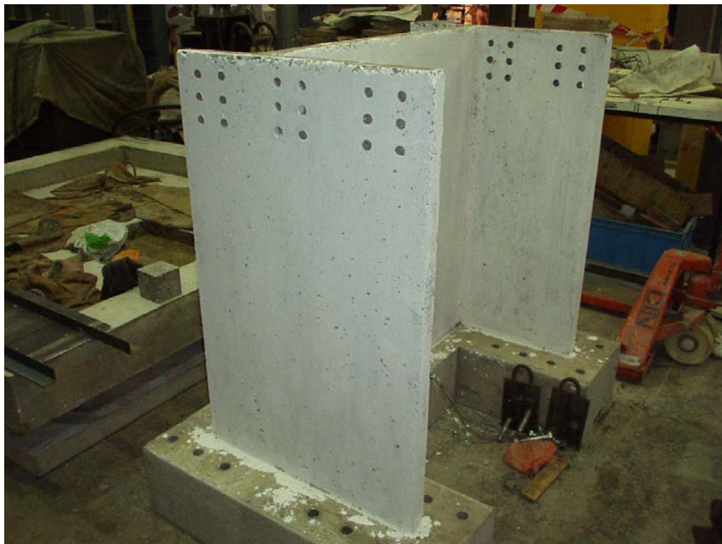
Figure 4.27 3D view of the wall model after white wash
