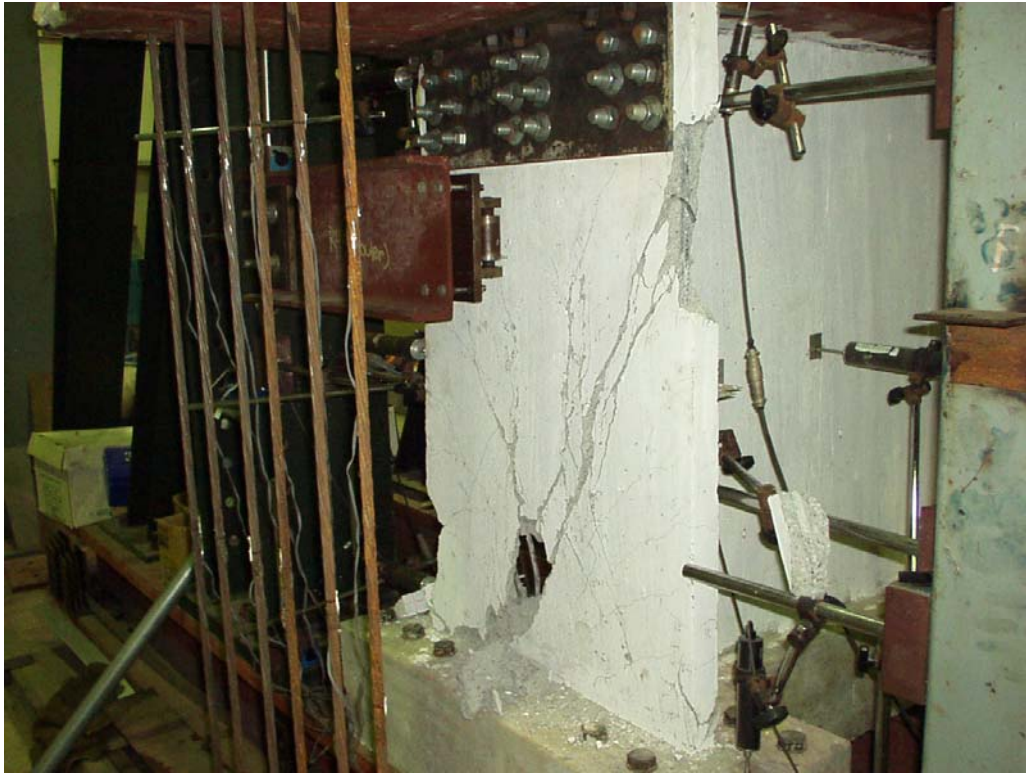
Figure 4.30 Overview of the shear failure mode of the right flange wall
