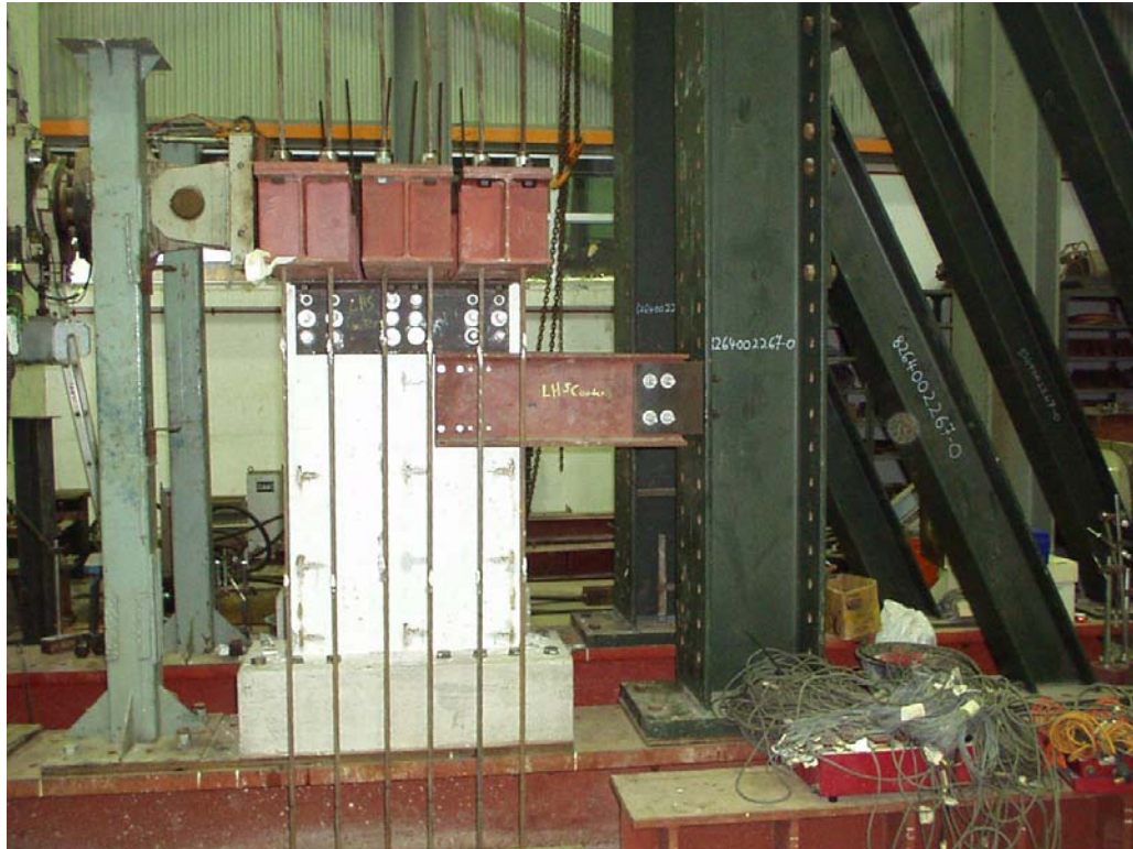
Figure 4.13 3D view of the overall test setup for the control wall (specimen S1)
