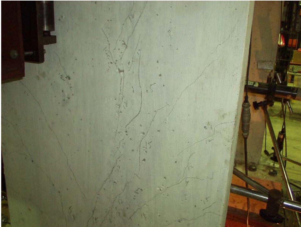
Figure 4.28 3D view of crack pattern of the flange wall
