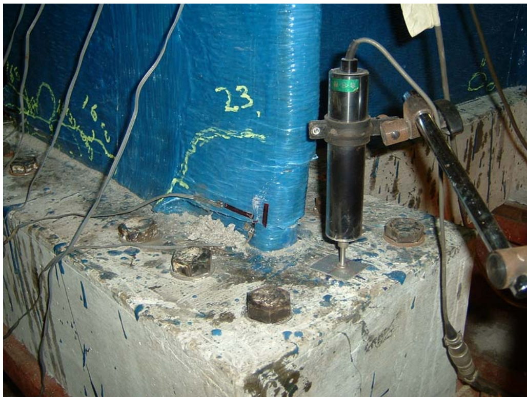
Figure 4.41 Crushing of the left flange wall
