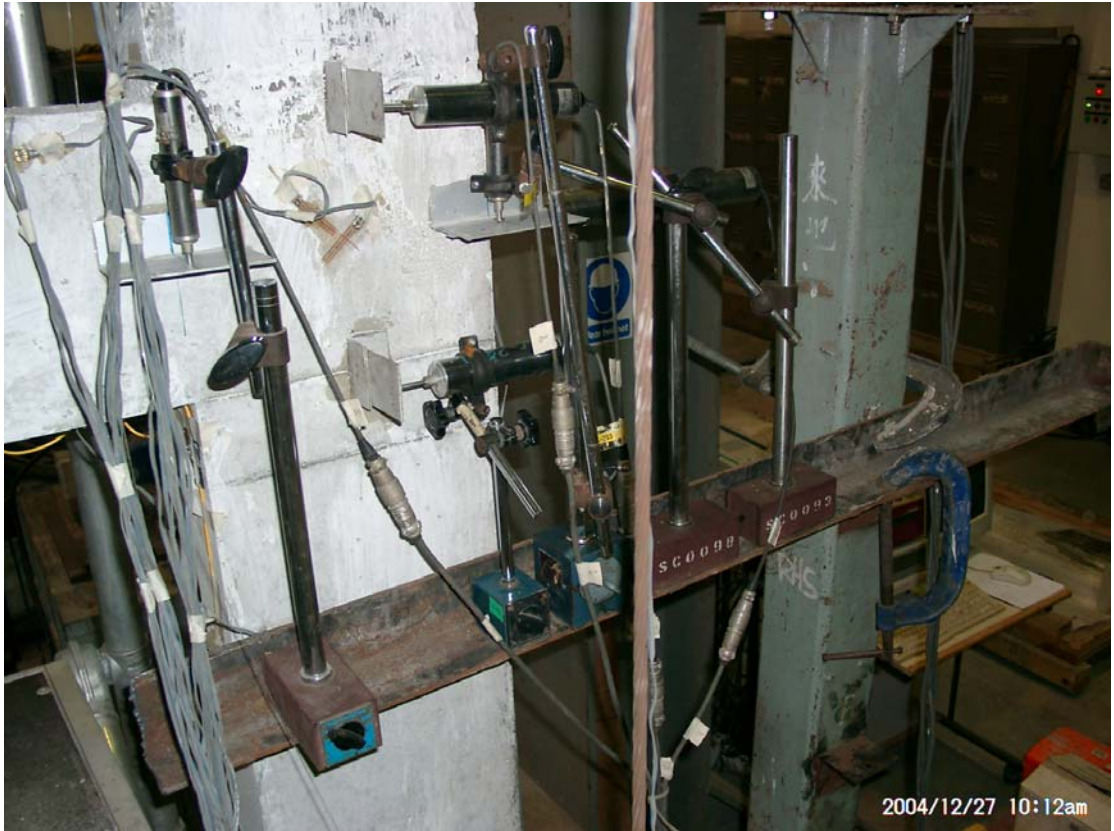
Figure 2.18 3D view of the transducers at the 1 st story external joint
