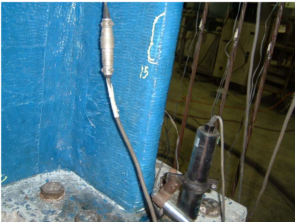
Figure 4.35 First FRP debonding of the left flange wall
