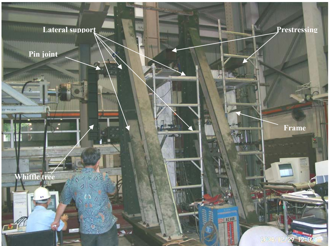
Figure 2.9 3D view of the test set-up
