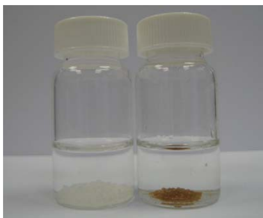
Figure 6.5. Images of CTS-MG before and after arsenate sorption in the presence of NOM
