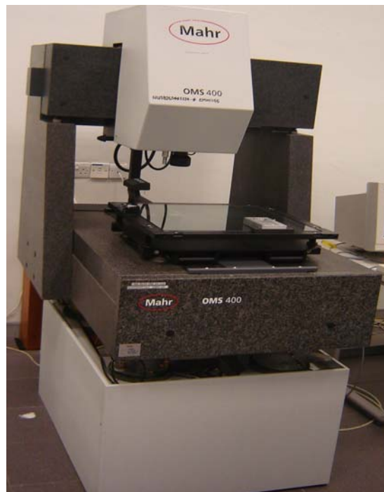
Figure 4.4: Picture of the Mahr OMS-400 CMM Machine
